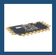
M2216 is a high-performance ultra-high frequency read-write module with 16 antennas for high-speed polling. It can be individually configured for power and time to meet different coverage requirements. The maximum output power of the module can reach+30dBm, coupled with an 8dBi gain antenna, the reading distance can reach 20m, and a tag recognition rate greater than 800tags/s can be achieved.
