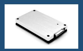
M2130 is an ultra-high frequency single channel read-write module designed based on PHYCHIPS PR9200. The maximum output power of the module can reach+30 dBm, and when combined with an 8dBi gain antenna module, the reading distance can reach 0-20m. It can achieve a tag recognition rate greater than 200 tags/s, and has stable multi tag reading and anti-interference capabilities.
