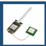
M2100 is an ultra-high frequency single channel read-write module designed based on PHYCHIPS PR9200. The maximum output power of the module can reach+25 dBm, and with an 8dBi gain antenna module, the reading distance can reach 6m. It can achieve a tag recognition rate of over 200tags/s, and has stable multi tag reading and anti-interference capabilities.
