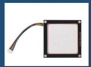
F90A1-S is an ultra-high frequency integrated read-write module designed based on PHYCHIPS PR9200. The maximum output power of the module can reach+25 dBm, and it is equipped with a 1dBi circularly polarized ceramic antenna. The reading distance can reach 2.5m and the tag recognition rate can be greater than 200tags/s. It has stable multi tag reading and anti-interference ability.
