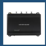
F5860-H is a **four port** UHF RFID fixed reader, which embeds the M2240 module. Its communication interfaces can be USB, RS485, RS232, and 100M Ethernet, etc.. It has four TNC antennae interfaces. Aluminum alloy of the whole body makes this reader more rugged and durable as well as the excellent heat dissipation capability, antijamming capability and lightning-proof ability.
